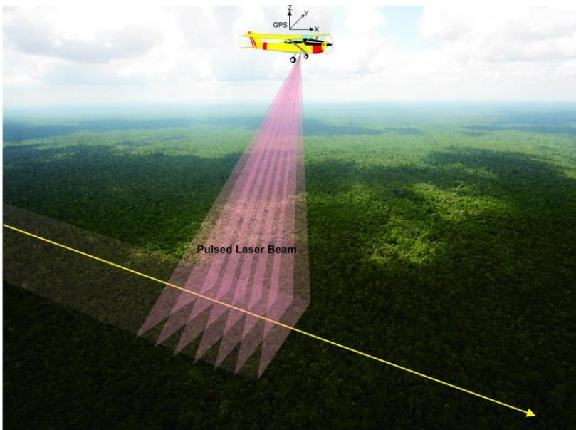
*Caption: Light Detection and Ranging (LiDAR) uses pulsed laser to generate precise three-dimensional information about the shape of the Earth surface elevation and vegetation. Such data are generally not available in Indonesia, and are needed for peatland management*
